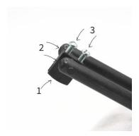
A small cross hole can be seen on the bottom of the head (1). Insert the cutter's fin into the slot on the bottom of the head. The provided head pin (a 19 brad nail) should be inserted through the hole, and the hole on the cutter. Once inserted, clip the pin to length.
